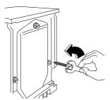
Remove the polystyrene base and take off the bottom panel by unscrewing the central screw.
